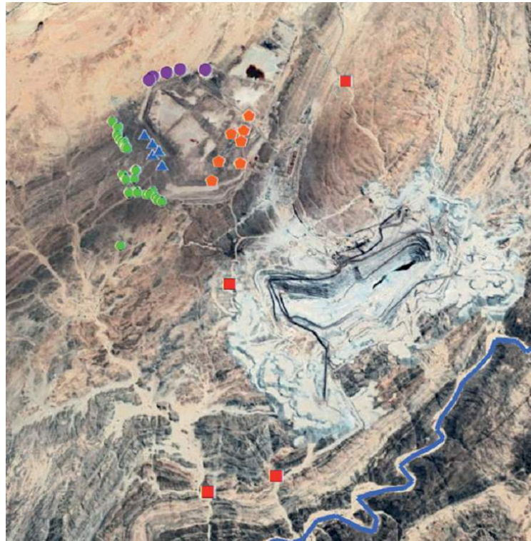
Figure 10: RUL seepage control pumping sites (NTSC in purple circles, TDDS in blue triangles, TDX in orange pentagons, DW in green circles & TRENCHES in red squares) and Khan River (blue solid line).
