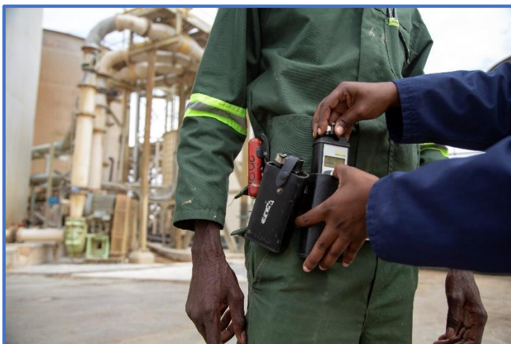
Figure 2: A worker wearing radiation monitoring instruments
