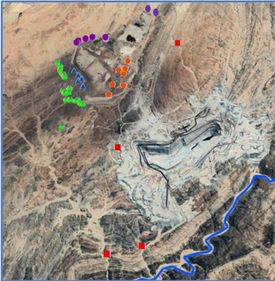
Figure 11: RUL seepage control pumping sites (NTSC in purple circles, TDDS in blue triangles, TDX in orange pentagons, DW in green circles & TRENCHES in red squares) and Khan River (blue solid line).
