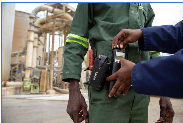
Figure 2: A worker wearing radiation monitoring instruments
