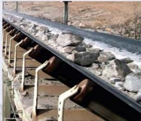
**In the existing Ore Sorting Pilot Plant, the material is scanned for radioactivity. Only radioactive material is accepted. Waste rock is ejected for disposal.**
