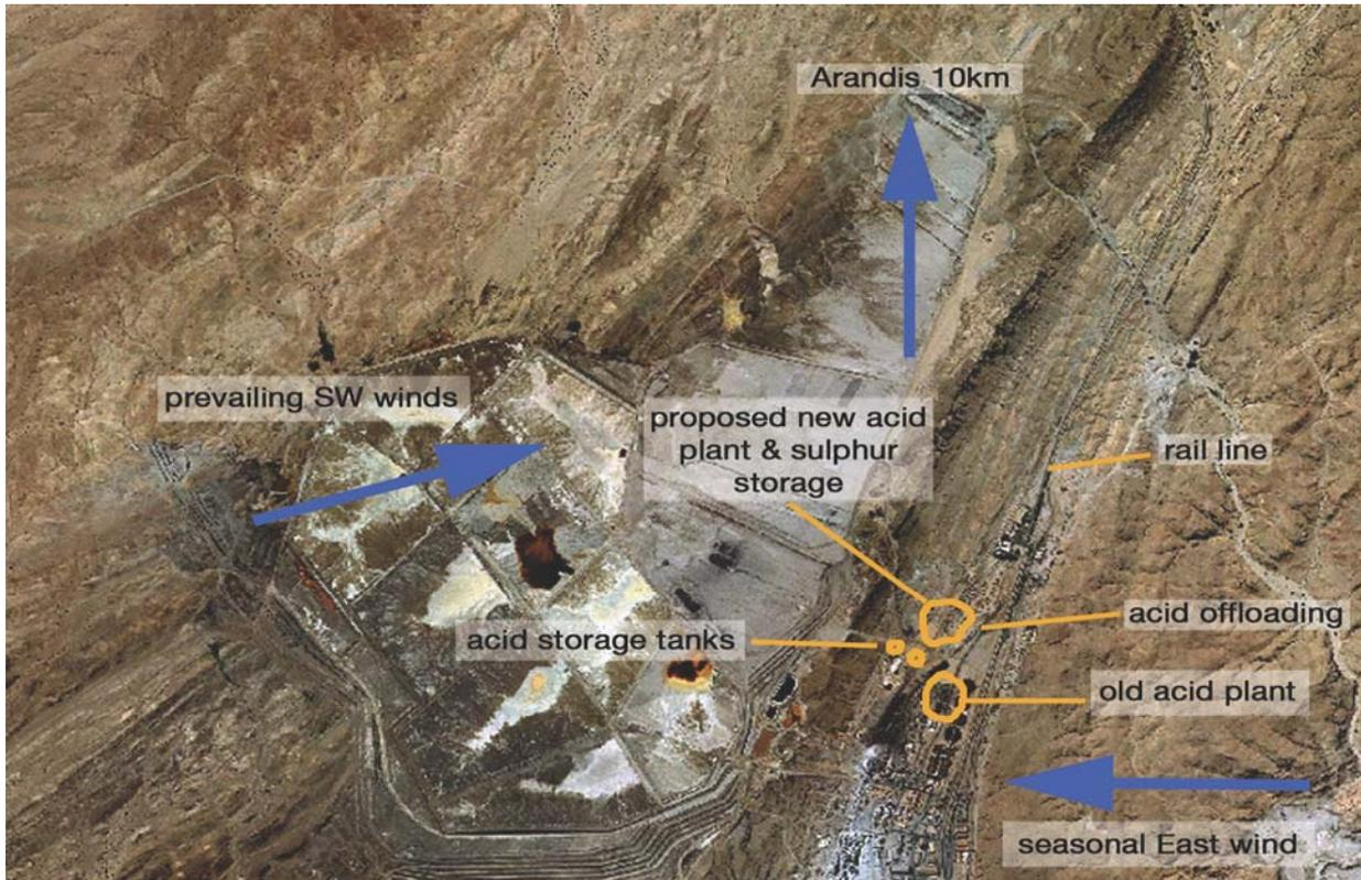
**Figure 10: Overlain on an aerial photograph, the proposed location of the new RUL acid plant relative to the old acid plant and other related sulphuric acid producing infrastructure** (source: RUL public participation material, 2007)
