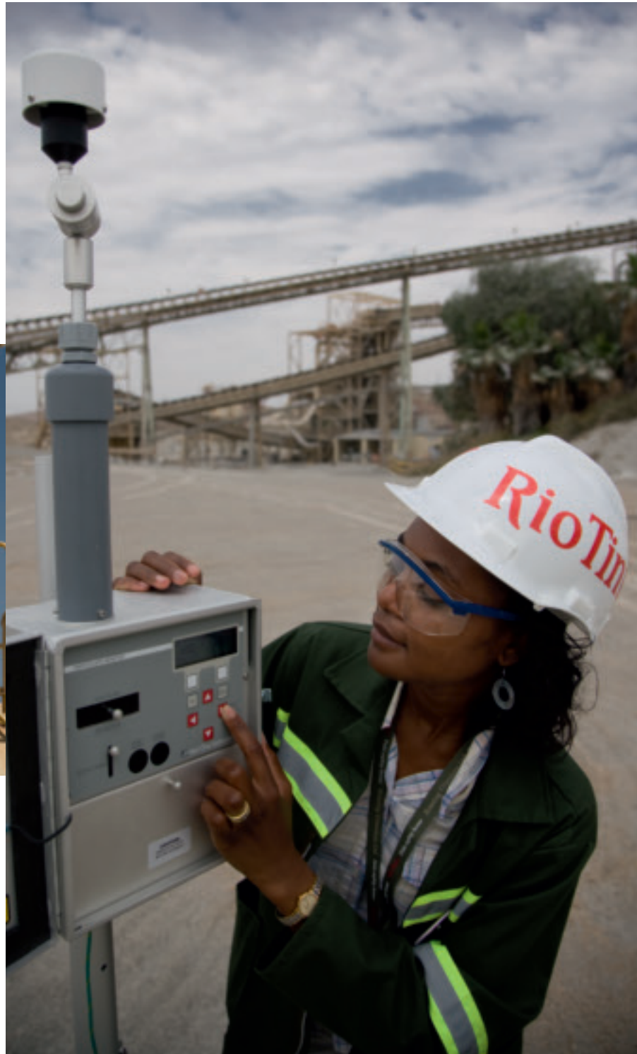
Above, environmental specialist Aina Kadhila Amoomo samples air quality at the crushing plant to ensure that levels of dust pollution are within acceptable limits.
