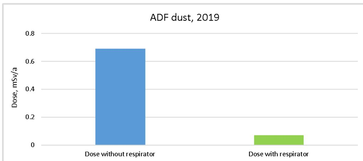
*Figure 7: Average dose rate for the automated drum filing area for 2019*
