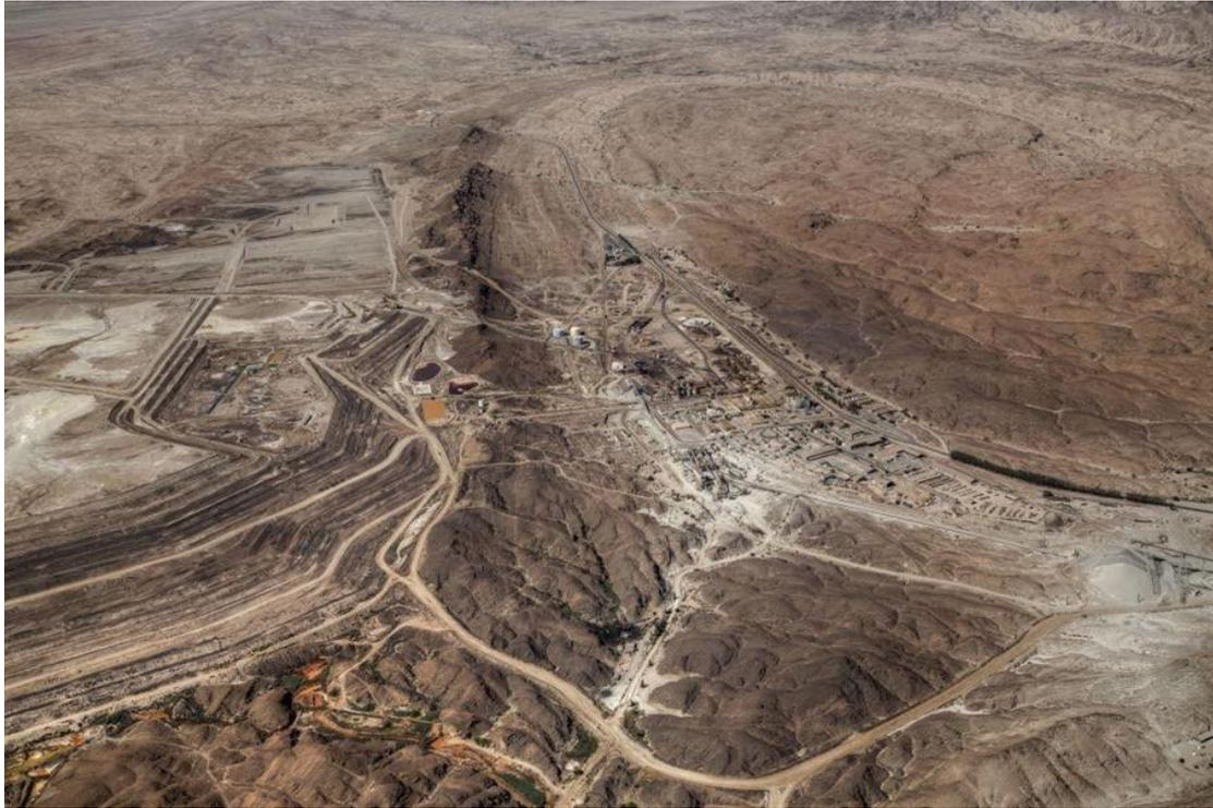
*Figure 8: Rössing’s TSF with seepage appearing at the bottom toe of the dam. The view is towards the North. (Photo: Karl-André Terblanche)*
