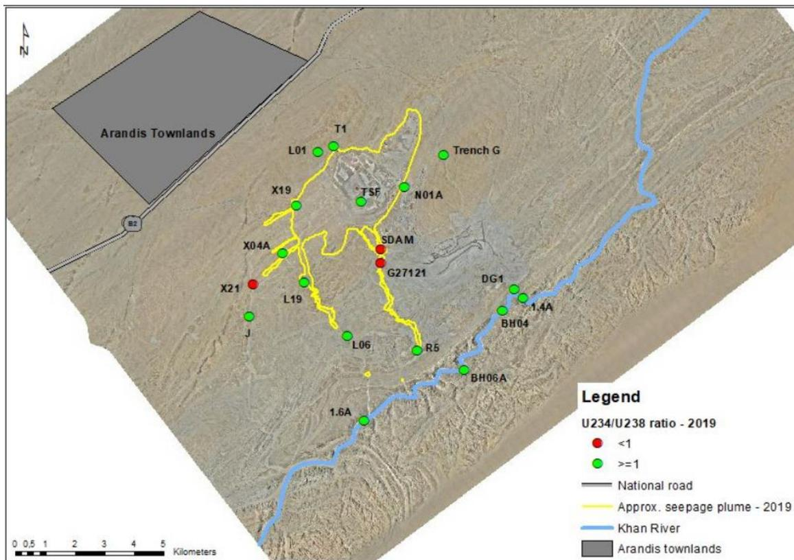
**Figure 10: Delineation of the seepage plume based on the sulfate method (yellow line). The two methods do not correlate at X21 and TSF.**
