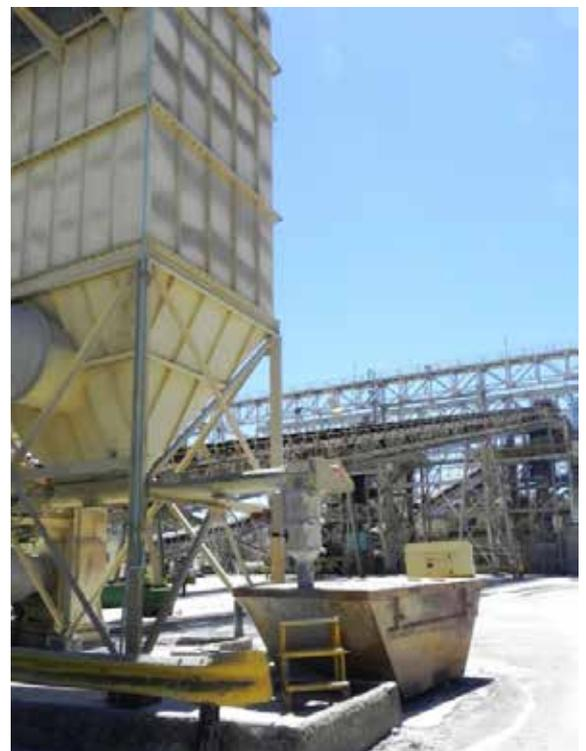
Figure 20: Fine crushing dust collection system
