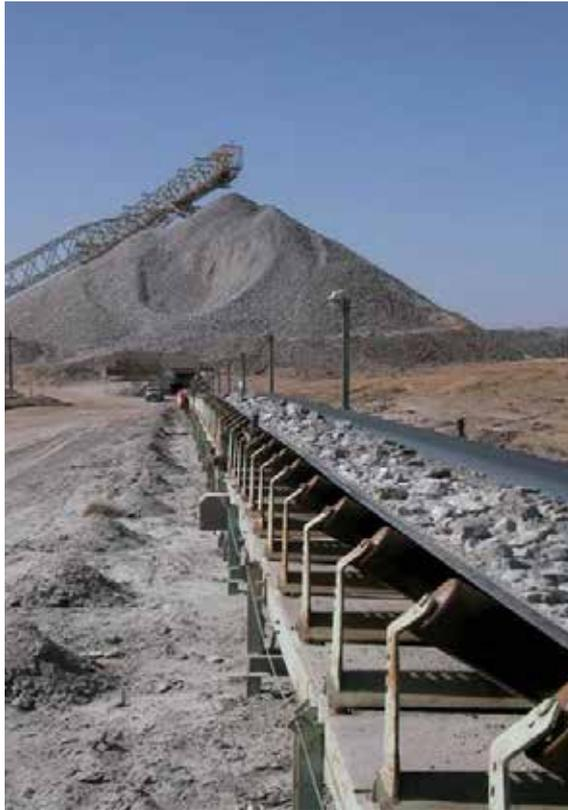
size. A conveyor belt transports the crushed ore to the Coarse Ore Stockpile (Figure 5) with a live capacity of some 80,000 tonnes. Coarse ore is withdrawn from the stockpile by vibrating pan feeders below the stockpile, feeding directly onto a coarse ore reclaim conveyor. This conveyor discharges the ore to a pre-screening plant where all fines are removed and the coarse material returned to the surge bin ahead of the Secondary Crushers. The ore is further processed through secondary,
