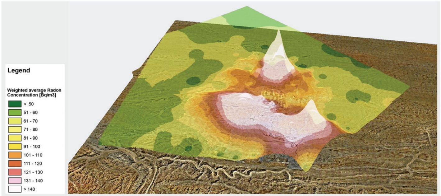
Figure 6: Three dimensional representation of radon concentrations at Rössing Uranium.
