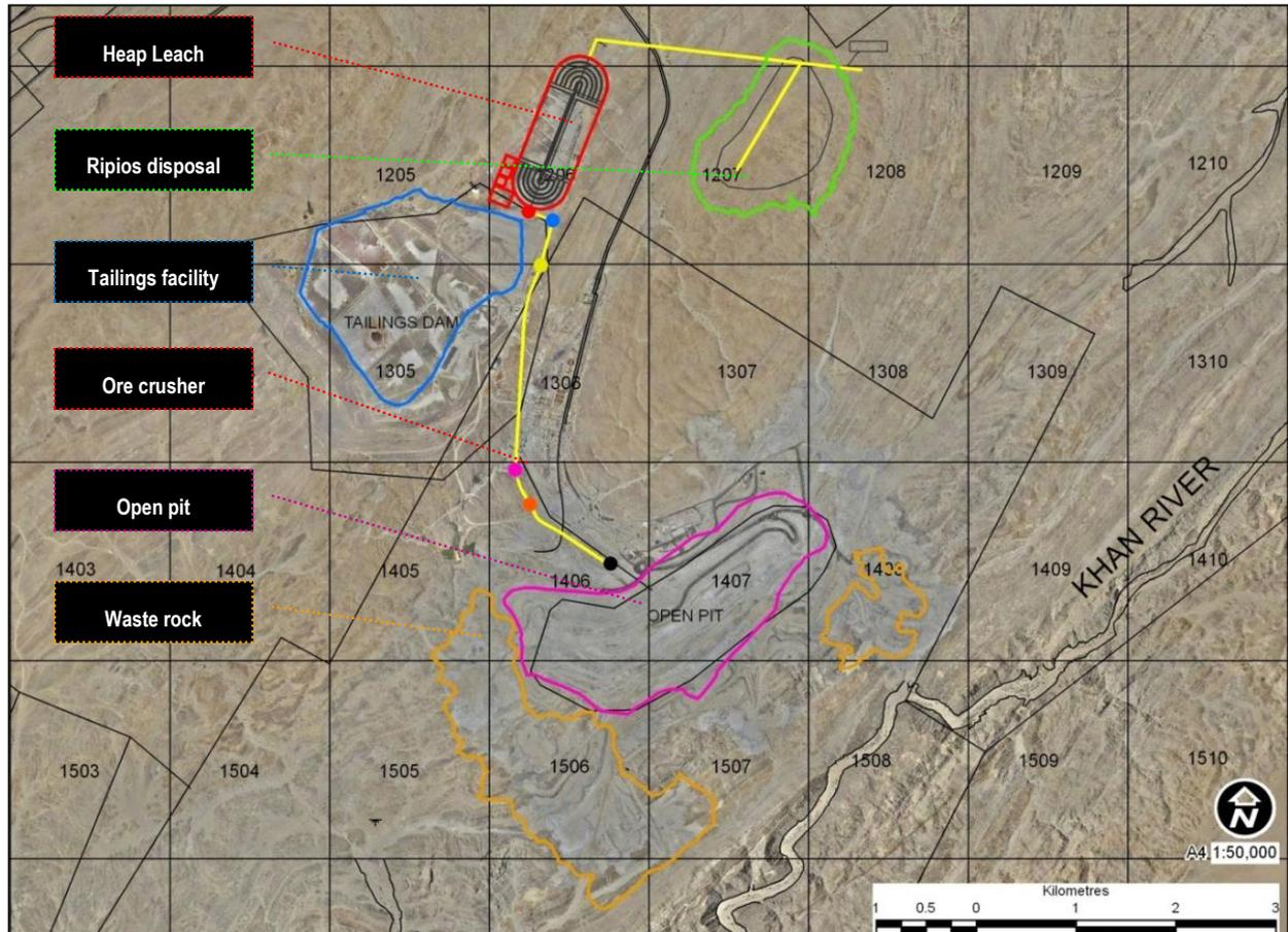
Figure 1: Overall layout of the mine expansion components being assessed
