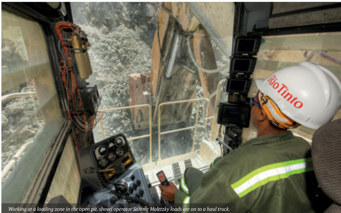
Working at a loading zone in the open pit, shovel operator Salome Maletzky loads ore on to a haul truck.
