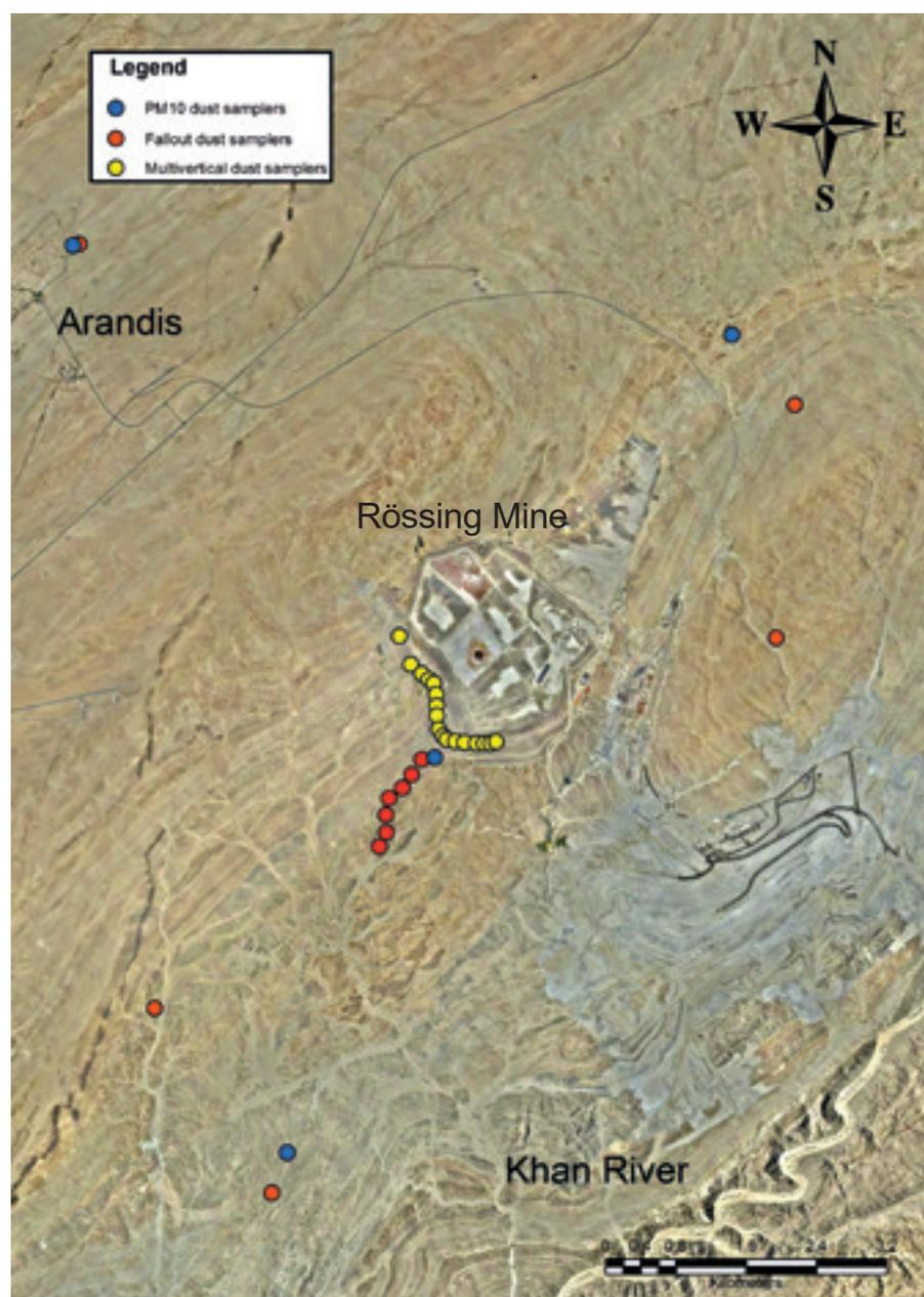
*A dust monitoring programme is underway to quantify the emission of total suspended dust from the Tailings Storage Facility during east wind events.*
