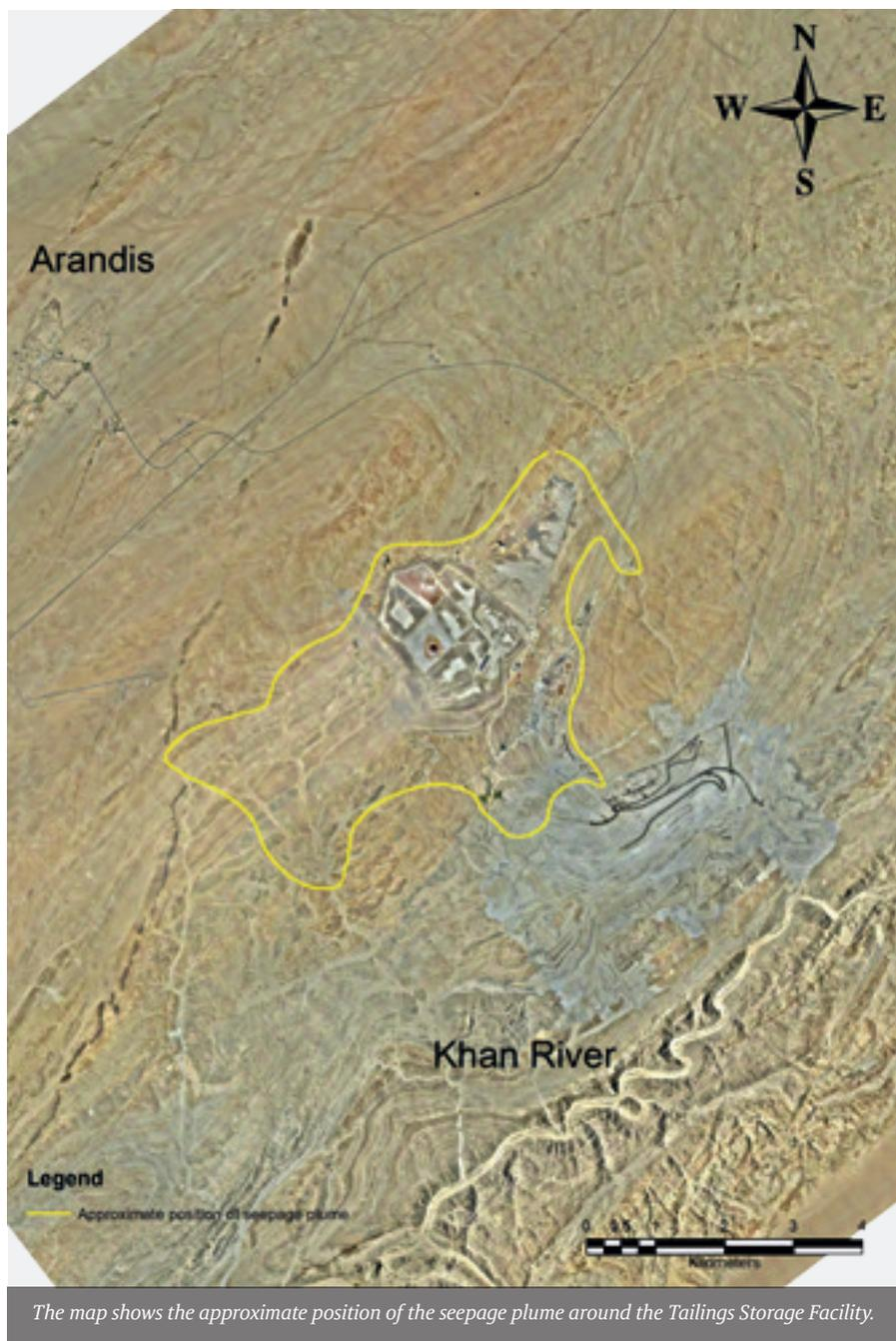
*The map shows the approximate position of the seepage plume around the Tailings Storage Facility.*
