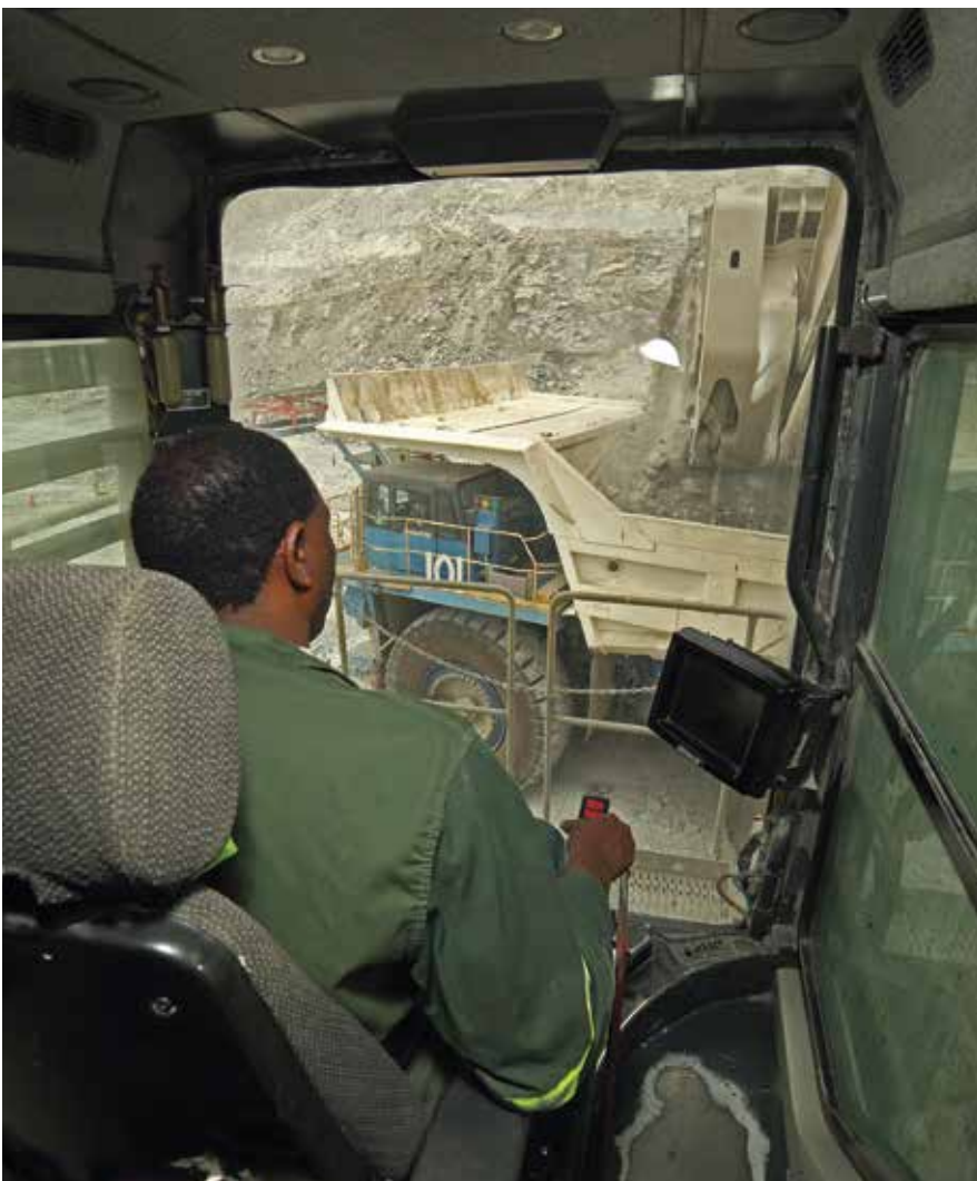
Shovel Operator Ndinoiti Vatekeuleni inside the cabin of a PC 5500 shovel in the open pit, loading a haul truck.
