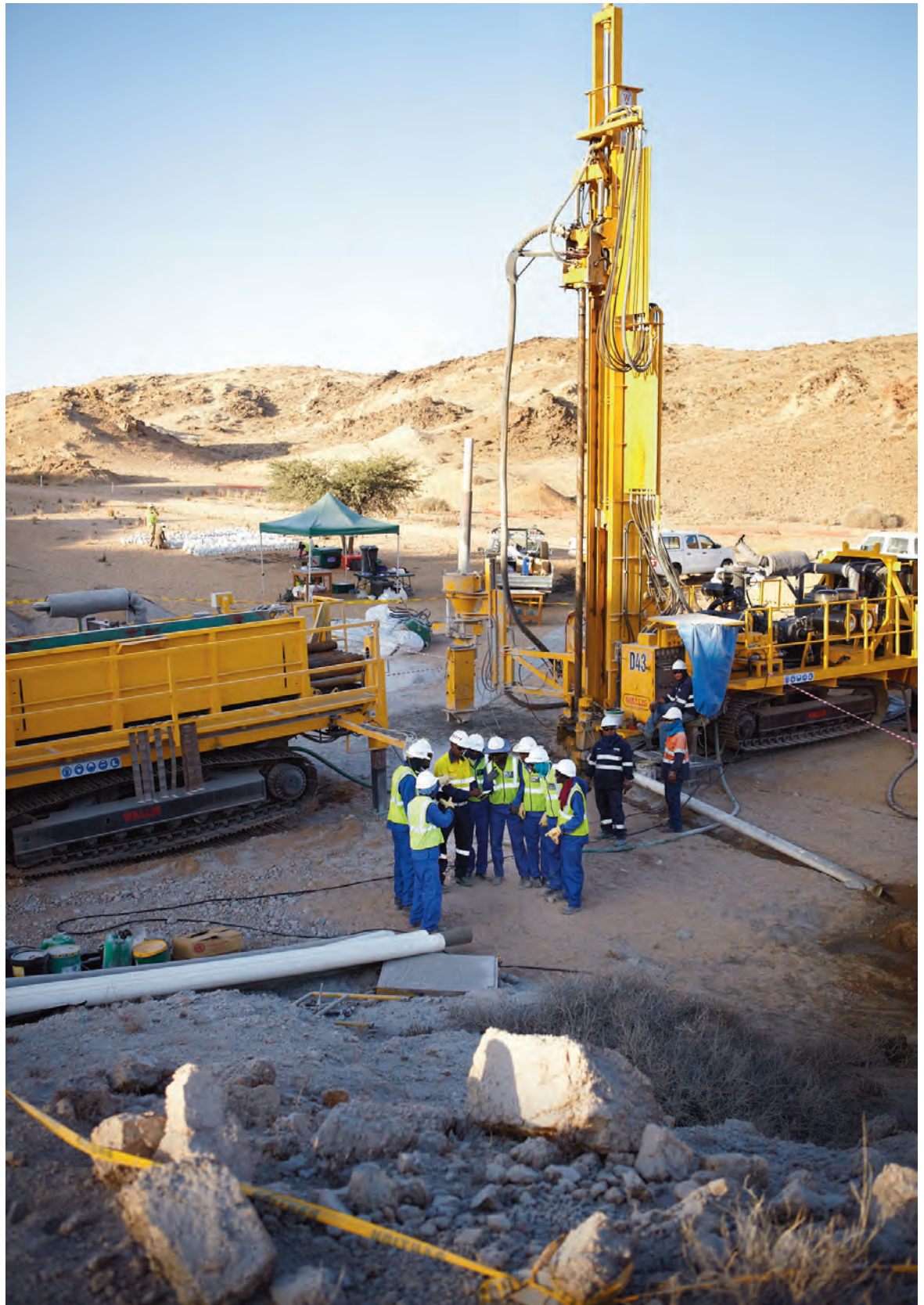
The reverse-circulation drill rig at the Z20 deposit where geologist Mesag Nekongo conducts a risk assessment with the contractor team.
