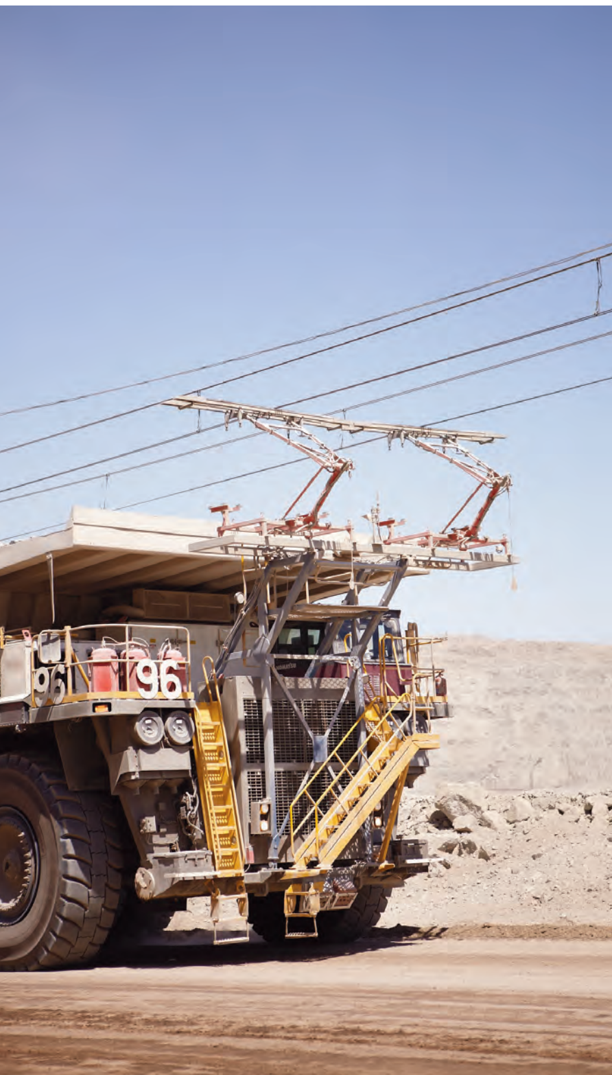
Haul truck 96 connected to Trolley line 13 as it drives on electricity from the loading zones in Phase 3 of the open pit.
