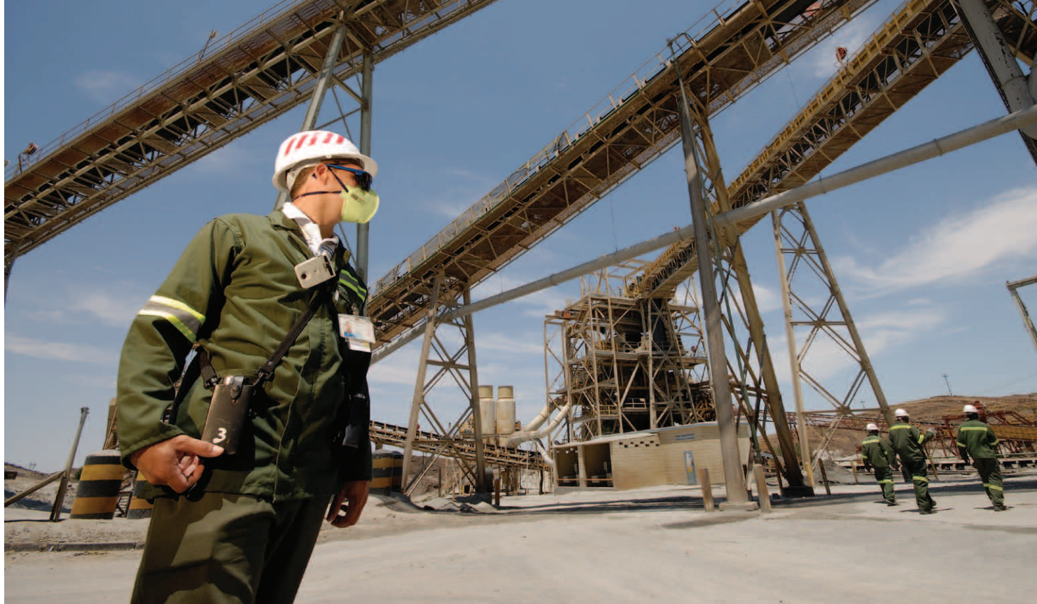
Juno Claasen, Radiation Safety Officer, in the Fine Crushing Plant, wearing a full set of monitoring instruments, i.e. a MyRIAM instrument (used for personal monitoring of radiation dose from the inhalation of dust), a DosemanPro instrument (used for personal monitoring of radiation dose from the inhalation of radon decay products), and a personal electronic dosimeter (used for monitoring personal exposure dose to external radiation).
