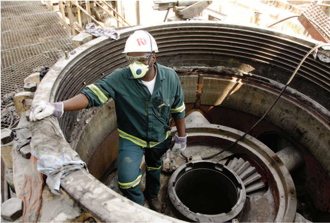
Malakia Povanh, Fitter, cleaning the mainframe bore area on one of the cone crushers of the tertiary crushing section at the Fine Crushing Plant.
