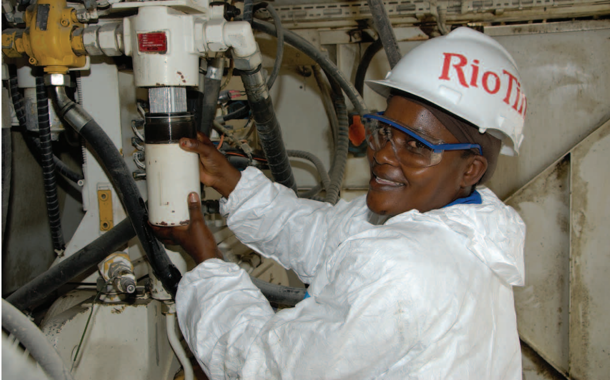
Fiina Kuutondokwa, the only female Fitter in the Mining Department, changing an oil filter in one of our shovels operating in the open pit.
