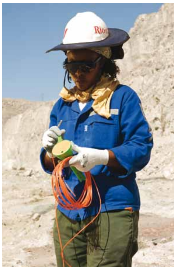
Aretha Mutumbulwa, a member of the blasting team, preparing for another blast to loosen the rock. She is busy priming a hole where the dynamite will be placed, holding a booster and a Nonel detonator in her hands.
