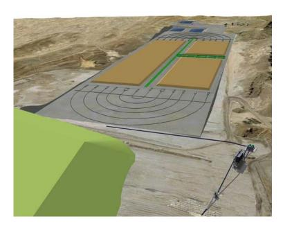
In addition, drilling of existing and new areas surrounding the current open pit has been undertaken to investigate the extent of the uranium ore available within the Rössing mining licence area. The expansion will result in an increase in size and depth of the current open pit, which in turn will require larger waste rock dumps and tailings facility.
