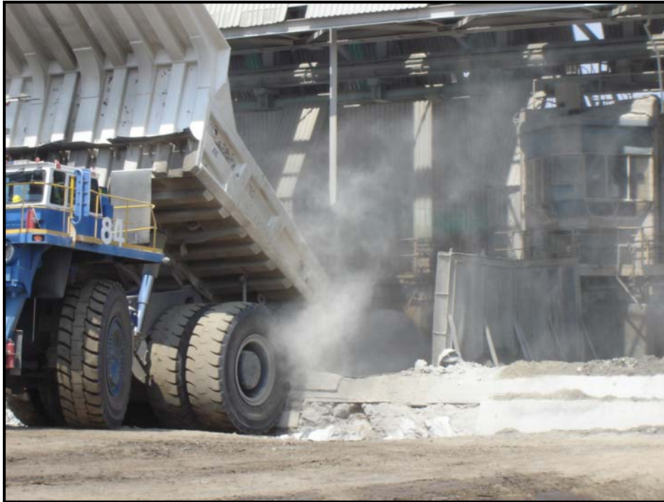
Figure 4-9: Truck tipping ore.
