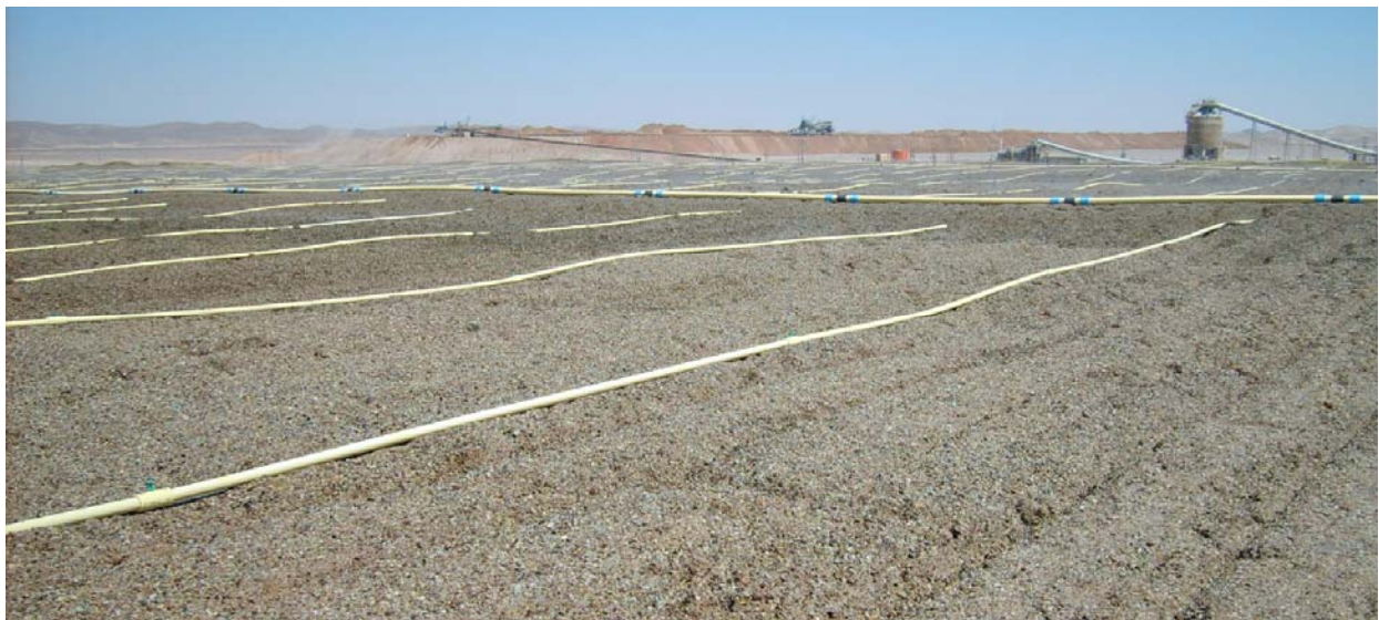
Figure 11: Example of an “on-off” layout for heap leaching (source: RU)
