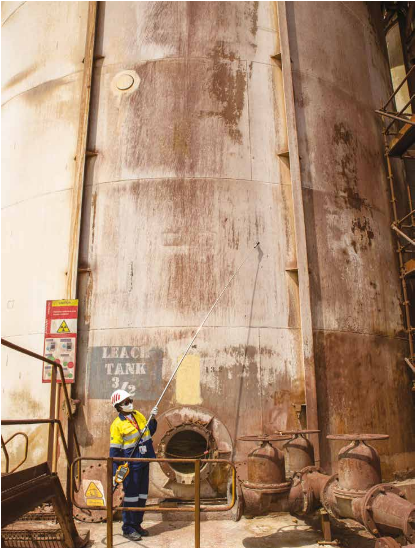
Nelao Endjala, advisor radiation safety, at one of the tanks in the Processing Plant, with an Automess Teletector Probe instrument which is used to measure levels of gamma radiation in hard-to-access places, such as inside tanks.
