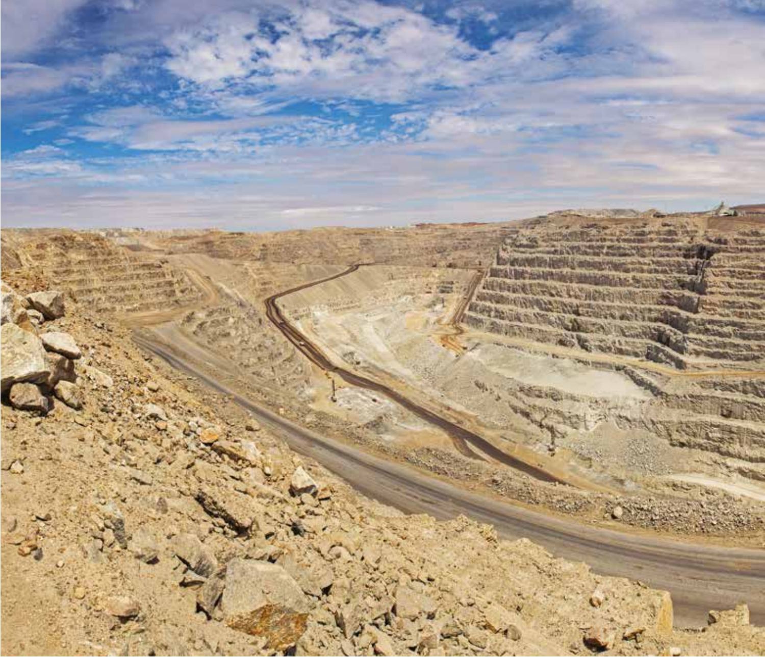
A view of the mine's open pit which currently measures 3 km long by 1.5 km wide, and is 390 metres deep.
