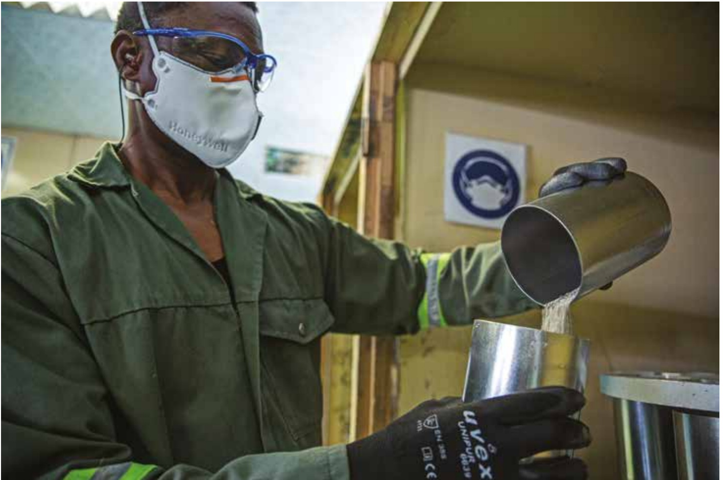
Laboratory technician, Cornelius Manjara, of the chemical laboratory at the mine is preparing a test sample from milled rock from the open pit.
