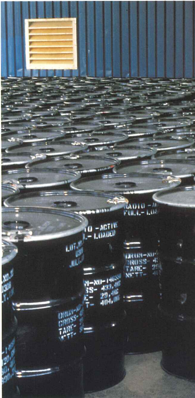
Rössing's final product, uranium oxide, is a powdery substance and is safely and securely packed into steel drums for delivery to the Company's customers. One drum of uranium oxide, which contains almost 400 kg, contains the equivalent in energy of 25 000 barrels of crude oil.
