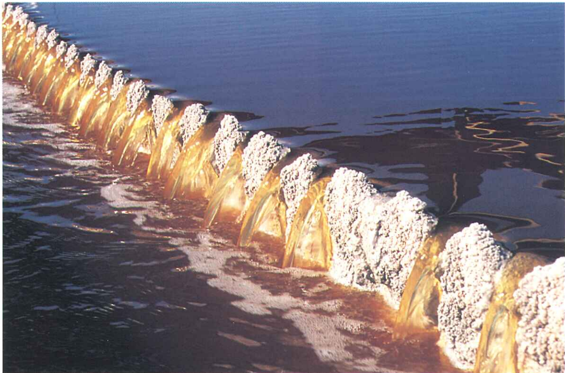
In the counter current decantation (CCD) tanks a flocculant is added to weigh down the slimes to the bottom with the clear uranium-bearing solution, also known as the pregnant solution, overflowing into a tank.
