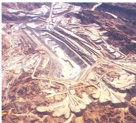
An aerial view of the open pit, which is 3km long, 1km wide and 300m deep.
