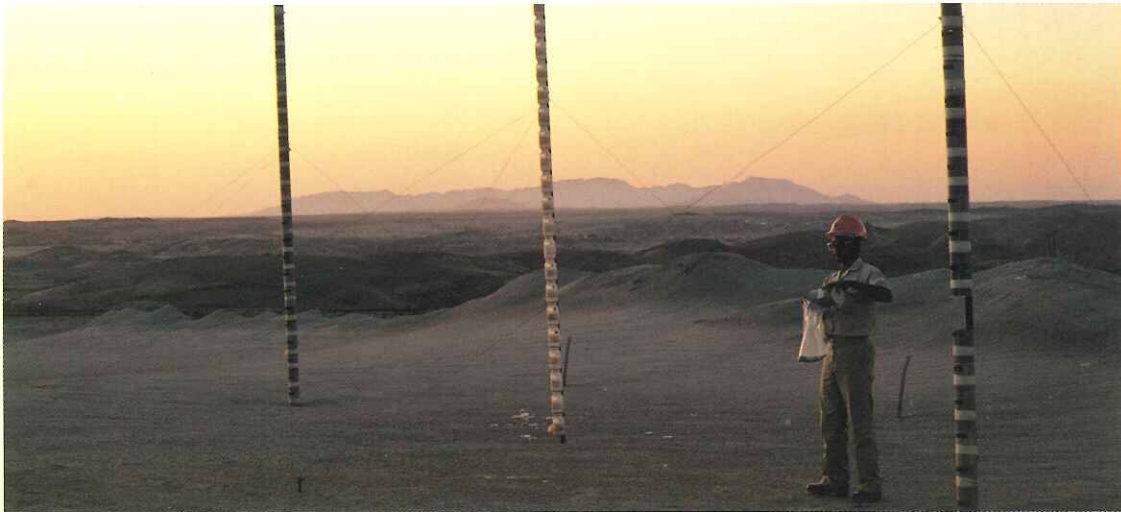
Various dust monitoring programmes are implemented to assess tailings erosion and to quantify the effectiveness of the control measures. The monitors used include the multi-vertical dust samplers, which have been designed by Rössing.
