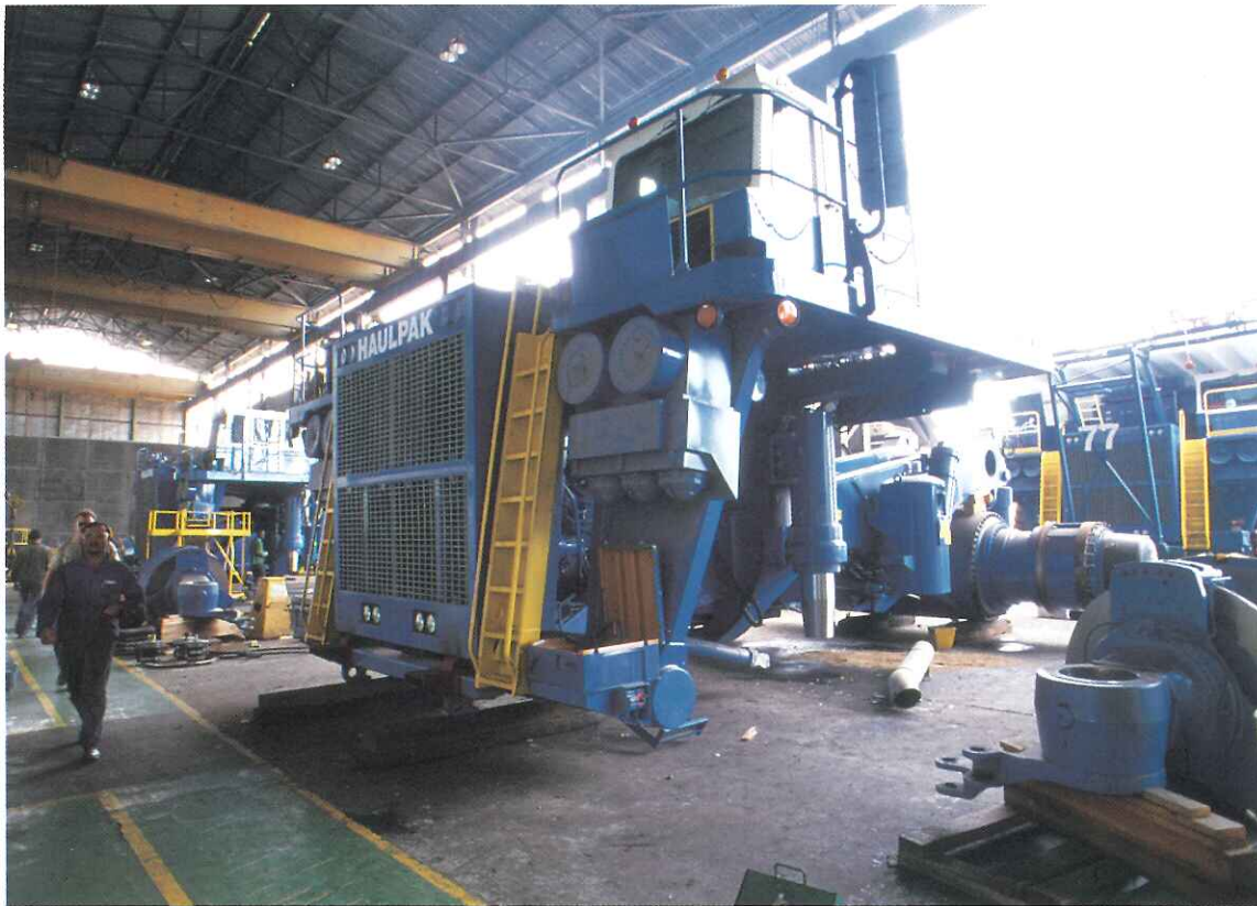
One of the five new 180 tonne Haulpak 730E haultrucks being assembled on the mine.
