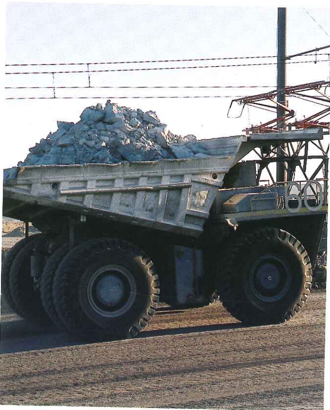
Haultruck on trolley assist
