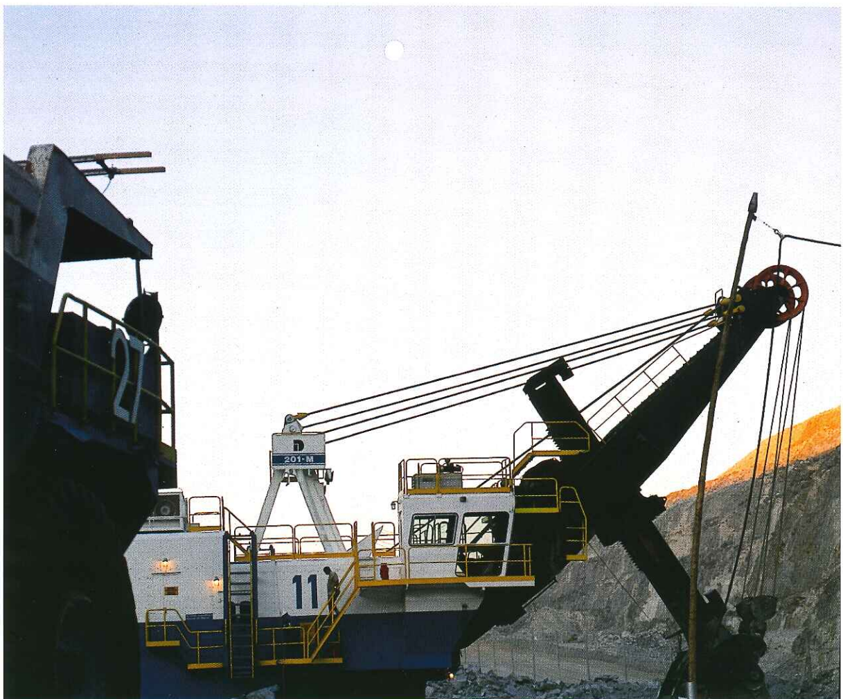
Rope Shovel at work in the Open Pit
