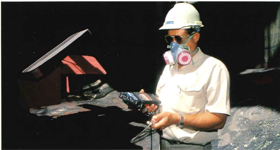
Checking for the presence of gas in a tank, as a precaution before maintenance work is done
