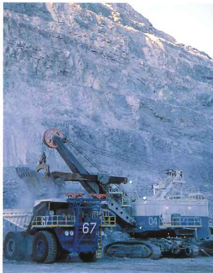
Loading a haultruck in the Open Pit
