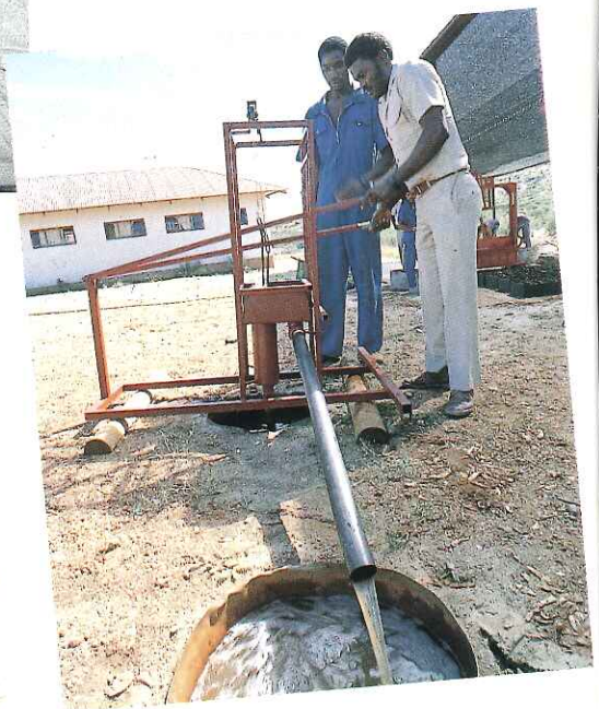
Third world technology at work. This hand (or foot) driven pedal pump, manufactured at the Brakwater Agricultural Training Centre near Windhoek, is ideally suited to the needs of rural farmers.
