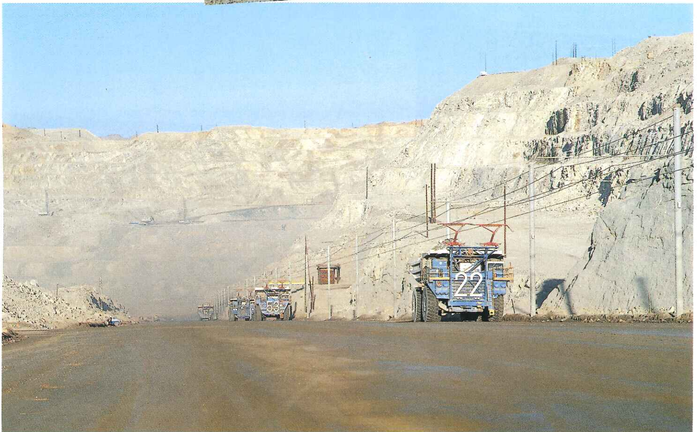
Haul roads in the open pit are continuously sprayed with water to reduce dust.
