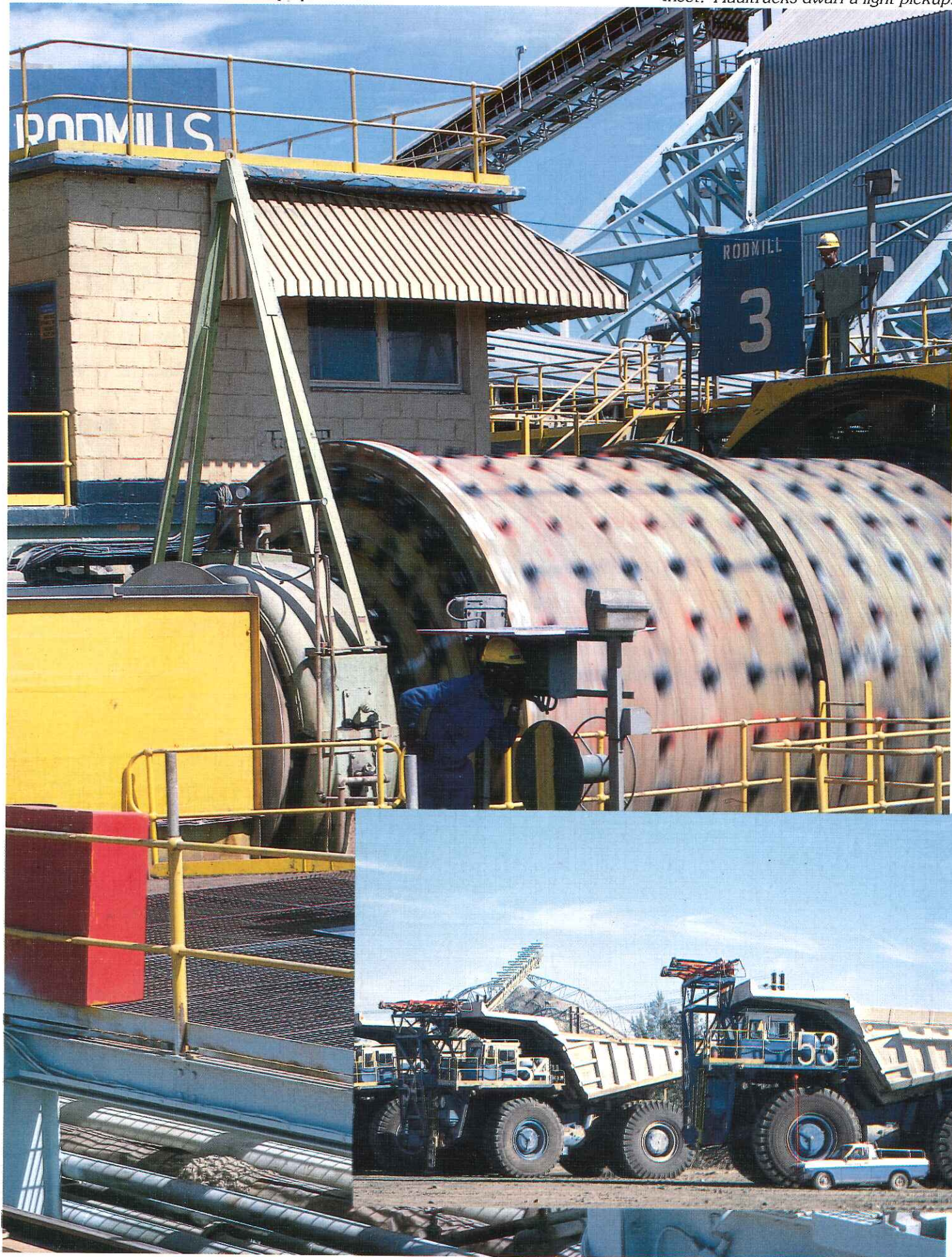
Rodmills grind the crushed ore to a pulp.
