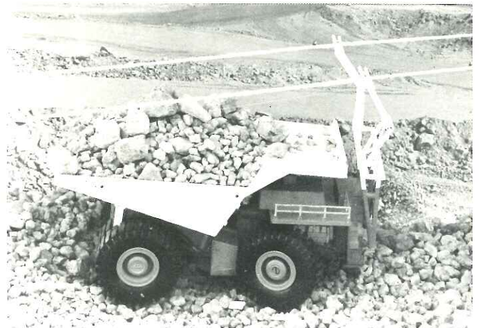
Scale model of a haultruck with overhead pantograph.
