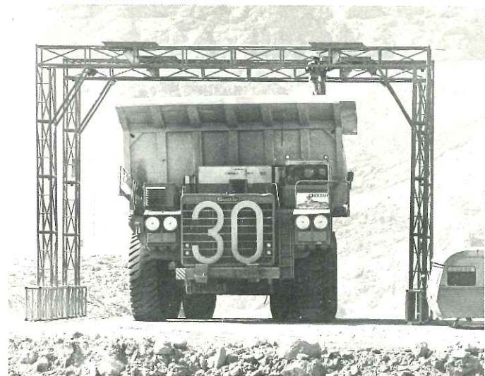
A haultruck passes under one of the ore-grade scanners.
