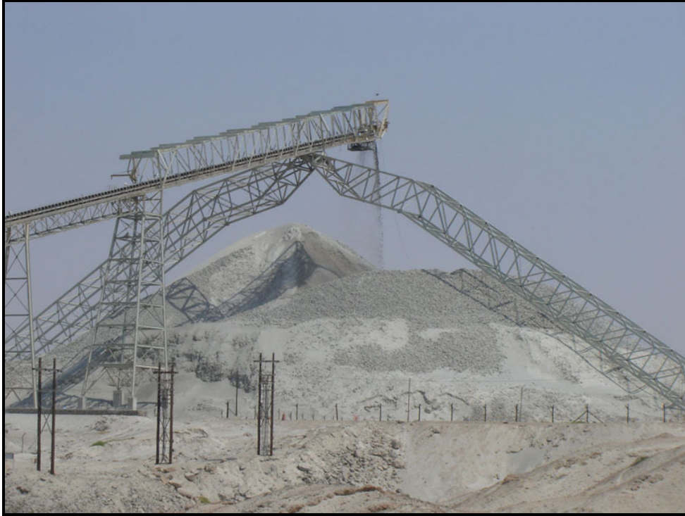
Figure 4-8: Tipping operations at the coarse ore stockpile (i.e. materials handling operations)
