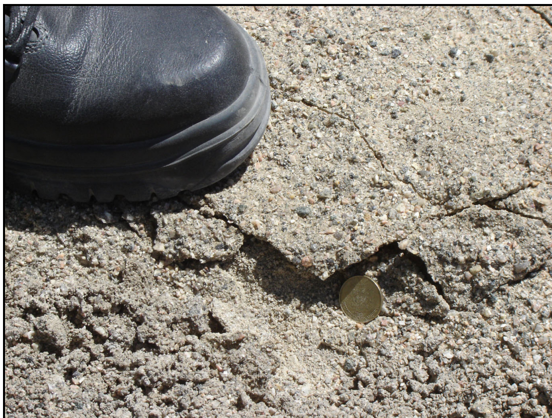
Figure 4-15: Crust formation on dry surface of tailings storage facility at Rössing mine
