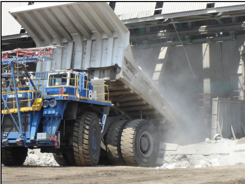
Figure 4-9: Off-loading operations at the primary crusher (i.e. materials handling operations)
