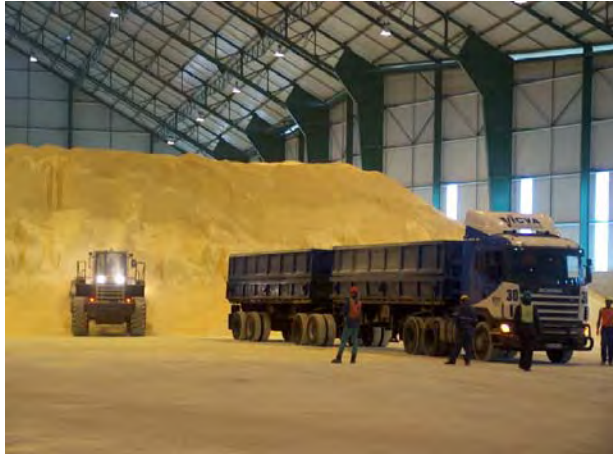
Figure 9: Typical enclosed sulphur storage shed 14
