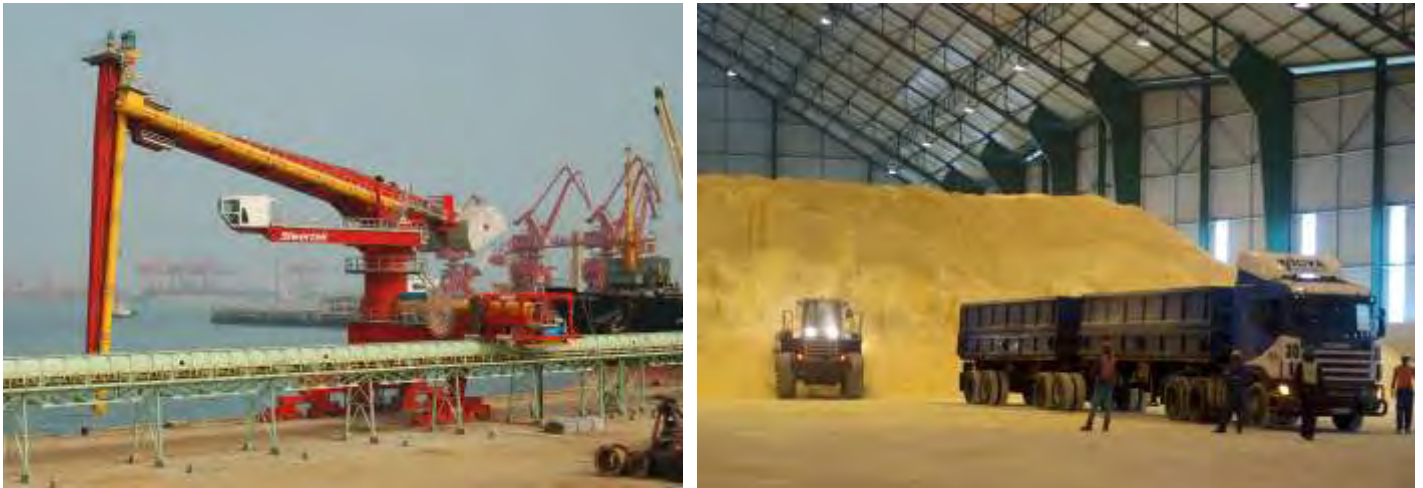
Figure 2: The illustrations above show a typical Siwertell ship unloader and a covered storage building as envisaged. Source: Ninham Shand Sulphur handling PID final. February 2008
