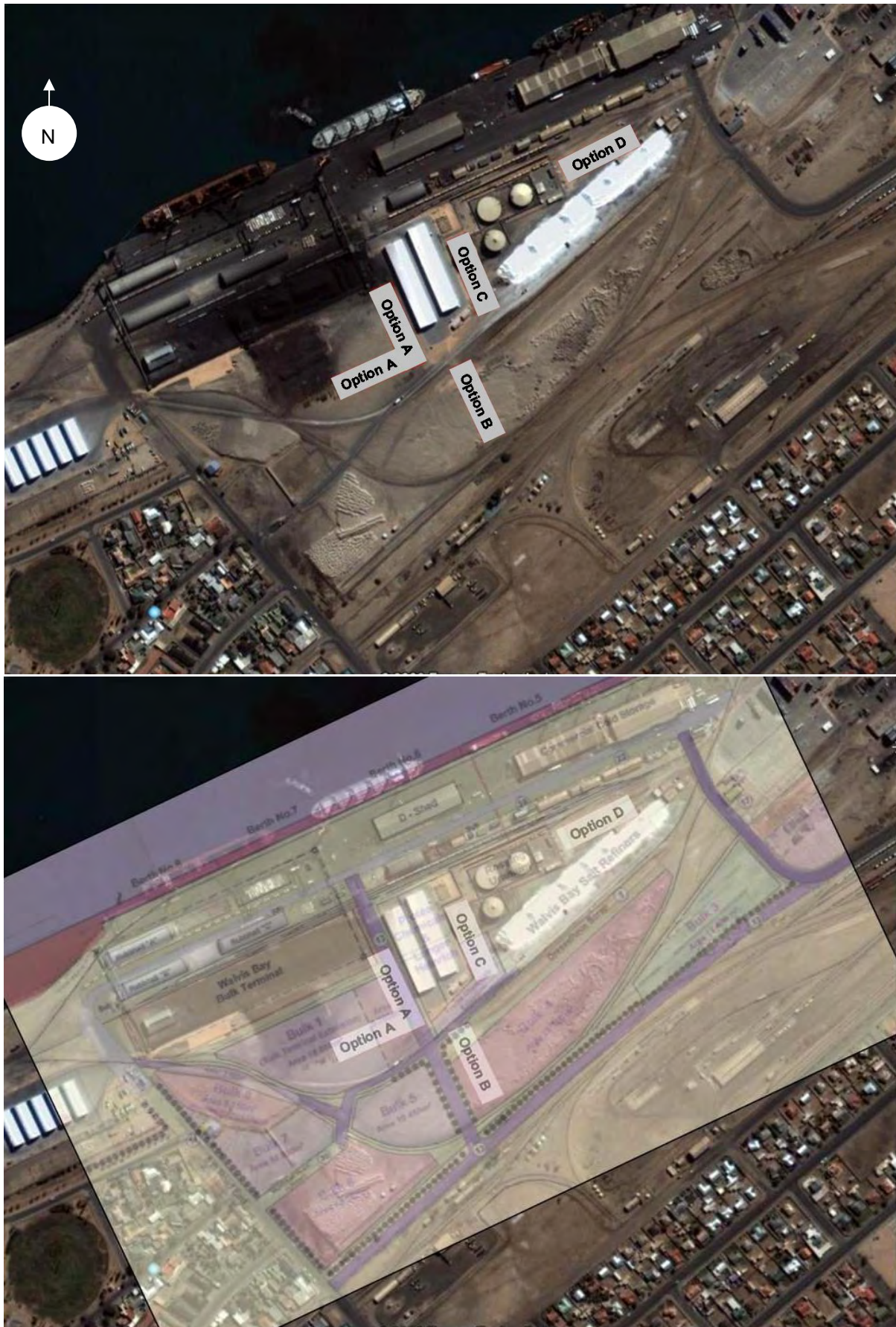
Figure 13: Site alternatives for the sulphur handling facility in Walvis Bay 19 and overlay with Figure 12: Port layout for comparison purposes
