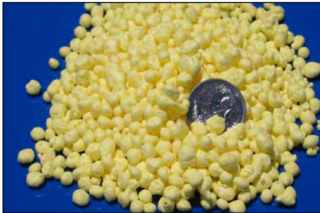
Figure 6: Elemental sulphur in prill form 11
