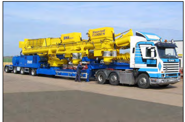
Figure 7: Mobile Siwertell ship unloader 12
