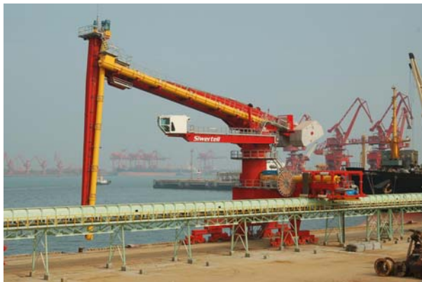
Figure 13: A typical Siwertell ship unloader and covered storage building (source: RU)
