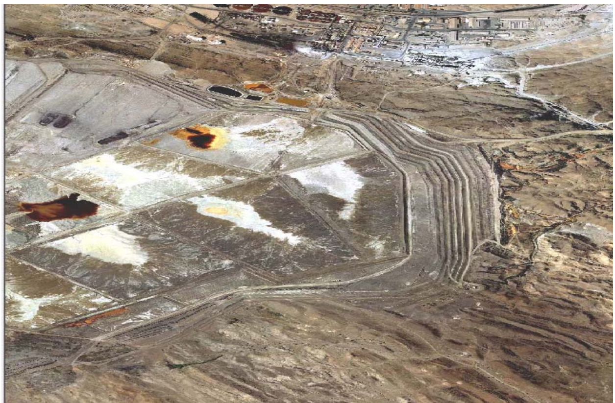
Figure 10: Current tailings dam design showing paddy system, viewed from the west (source: RU)
