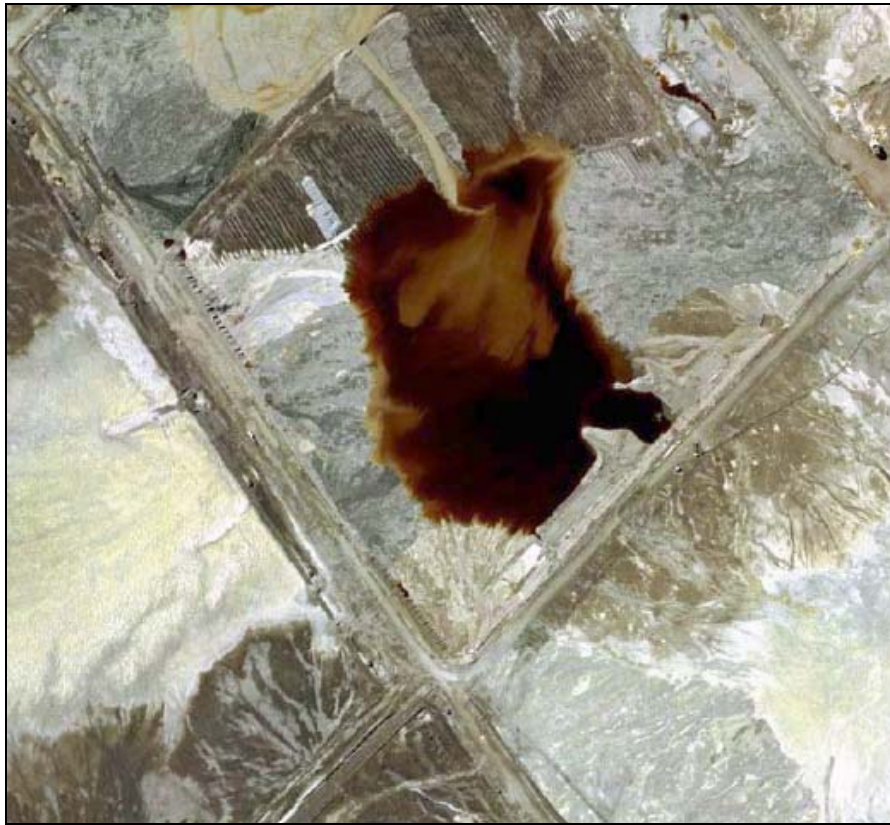
Figure 23: Tailings paddocks showing grey and yellow chemical precipitates after desiccation (source: RU)
