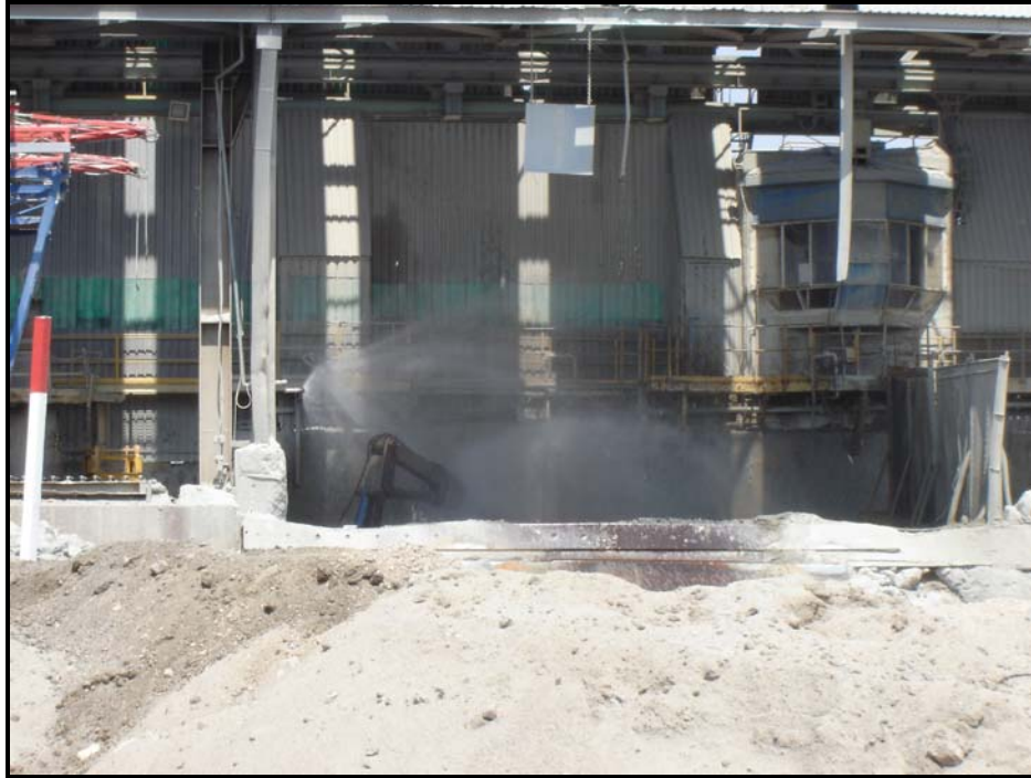
Figure 4-8: Water sprayers at the tipping site for the mined ore.
