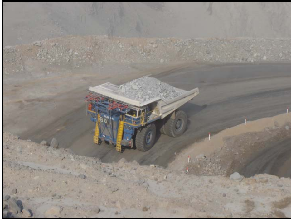
Figure 4-6: Vehicle activity within the pit travelling along a dusticided road surface.
