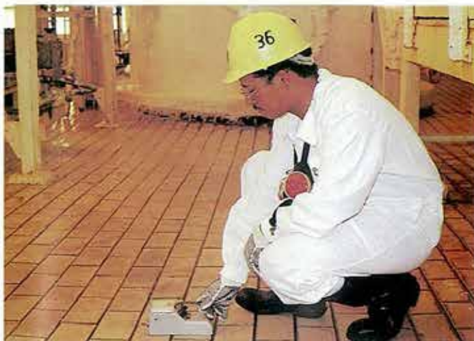
(C) An Environmental Officer taking radiation readings in the Final Product Recovery area.
