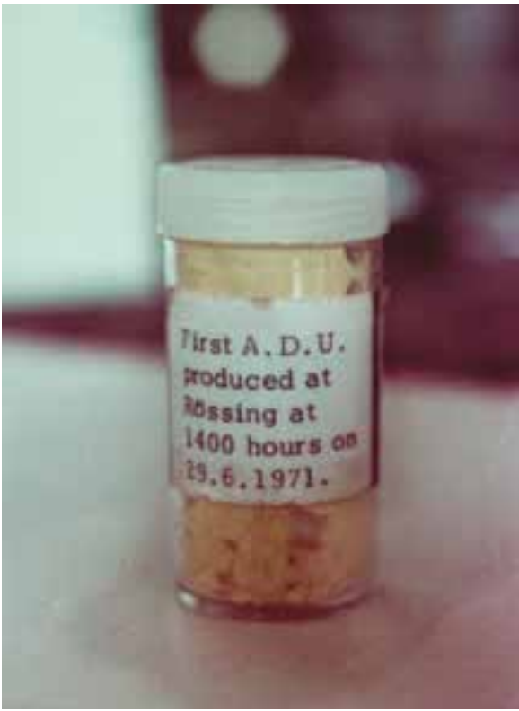
"First A.D.U. produced at Rössing at 1400 hours at 29.6.1971" Ammonium Di-urate (ADU) is the product of the precipitation reaction of OK liquor and ammonia. It is subsequently thickened, filtered and roasted to the finally produced U_3O_8 as the drummed product.
